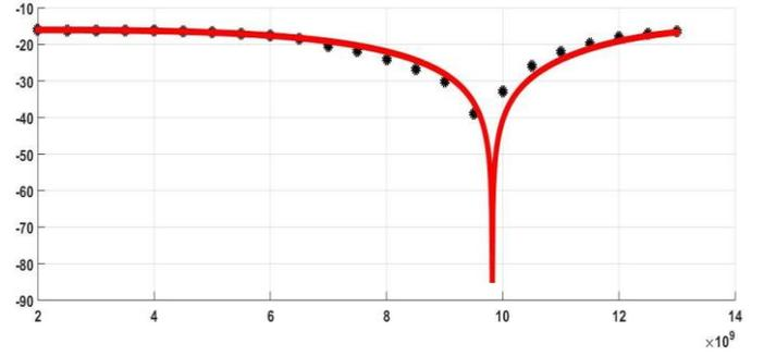
Figure 7. Simulated (line) and experimental results (dots) of power penalty depend on the frequency range between 2 and 13 GHz for the 40-km fibre length.
