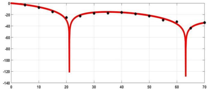
Figure 10. Simulated (line) and experimental results (dots) of power penalty depend on the optical length between 10 and 70 km for the 13-GHz frequency.
