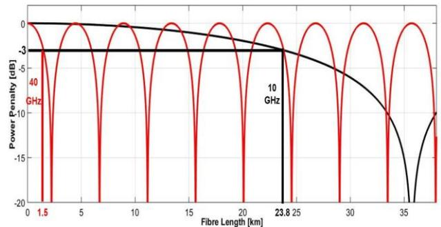
Figure 5. Power penalty of the oscillator signal depends on the optical fibre length.
