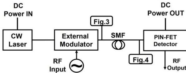
Figure 2. Analogue Optical Link with external modulator.
