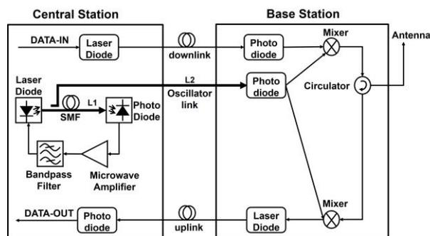
Figure 1. OEO implemented in the central station and connected to the base station with an analogue optical link.
