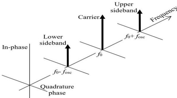
Figure 3. Spectrum of intensity-modulated optical signal at the modulator output at the fibre input.
