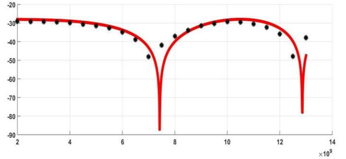
Figure 8. Simulated (line) and experimental results (dots) of power penalty depend on the frequency range between 2 and 13 GHz for the 70-km fibre length.
