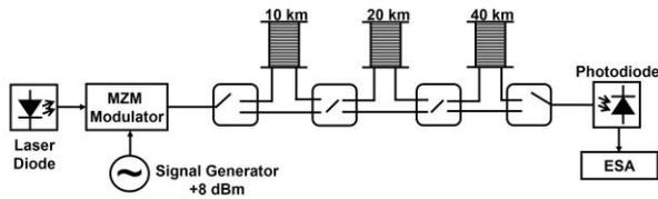
Figure 6. Experimental setup for the measurement on the analogue optical links.
