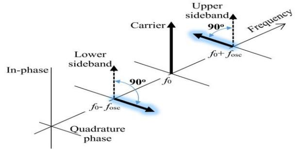
Figure 4. Worst-case situation for the spectrum of the intensity-modulated optical signal at the fibre output. Chromatic dispersion changes the phase relationship between the optical carrier and upper and lower sidebands to be of opposite phase.
