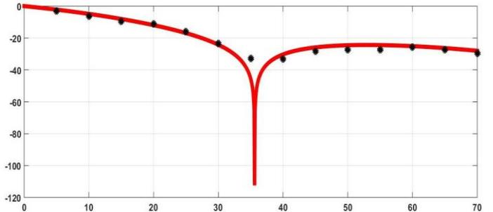
Figure 9. Simulated (line) and experimental results (dots) of power penalty depend on the optical length between 10 and 70 km for the 10-GHz frequency.
