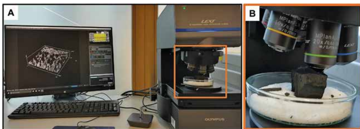
Figure 1. Charcoal observation: (A) Confocal Laser Scanning Microscope (CLSM) Olympus LEXT OLS5000 (Olympus Corporation Tokyo 163-0914, Japan), and (B) a detailed view of charcoal sample in a petri dish with table salt placed on the stage, under the objective of 20x magnification.
