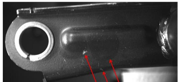
Fig. 4. Image A. A detail of a typical KTL-coated part with 3D form and black shiny color. Arrows point to the coating damage, dust and fingerprint.
