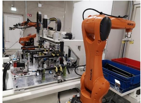
Fig. 2. Automated visual inspection system [8].
