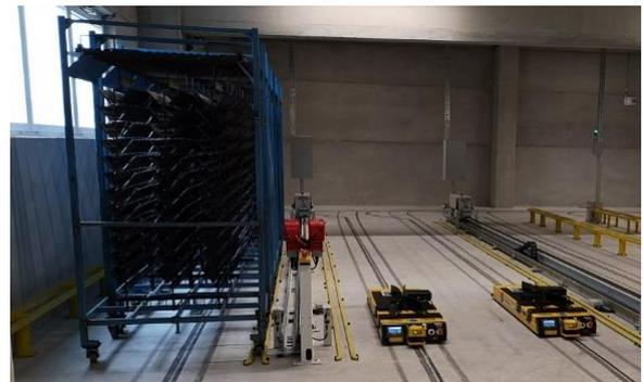
Fig. 3. Part transportation system with AGV-s.
