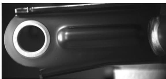
Fig. 5. The background image **B**. It is the average of a large number of images (>20) under the same lighting conditions and the same image acquisition setup.
