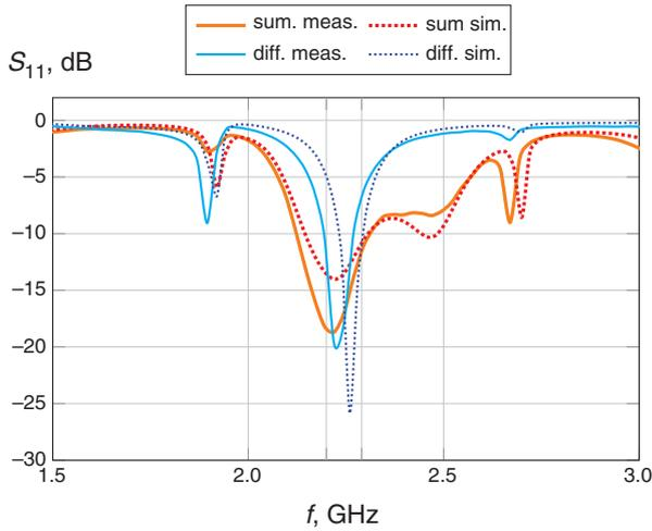
**Fig. 3** Impedance matching of both sum and difference ports
