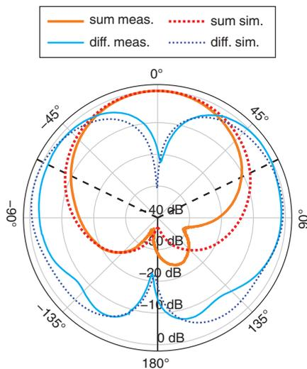
**Fig. 4** Radiation pattern in plane, perpendicular to sum balun
