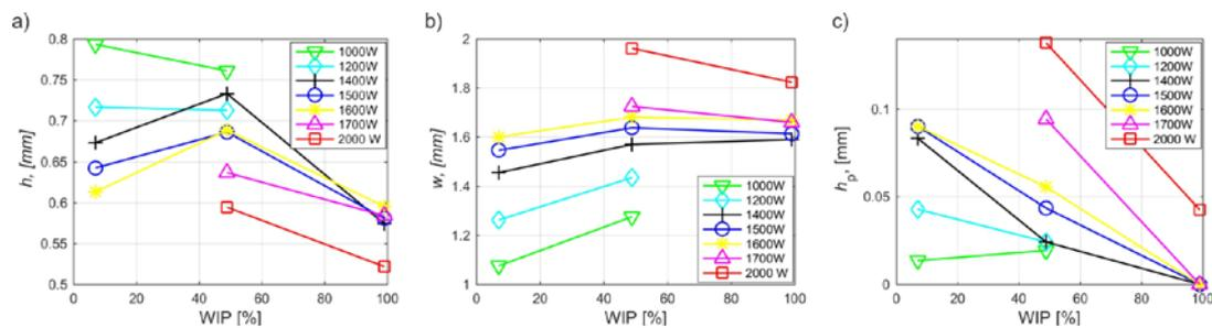
Fig. 5. Influence of the WIP at different values of the constant laser power  $P$  on a) the deposited layer height  $h$ , b) width  $w$ , and c) maximum penetration depth  $h_p$
