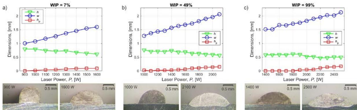
Fig. 4. Deposited layer height  $h$ , width  $w$ , and maximum penetration depth  $h_p$  at different values of WIP. a) WIP = 7%, b) WIP = 49%, c) WIP = 99%. Below the diagrams, photos of the layer cross sections at lowest and highest power  $P$  for each corresponding WIP value are presented.
