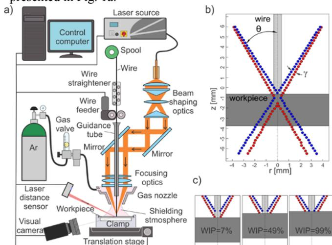
Fig. 1. a) Schematics of the experimental setup for annular laser beam LDWD, b) annular laser beam caustic, c) workpiece position at different WIP values.
