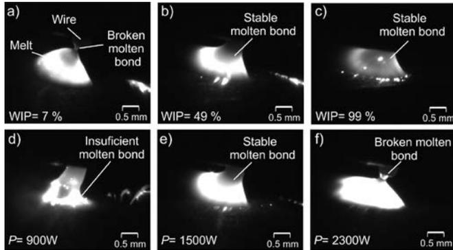
Fig. 2. Images of typical molten bonds taken during the LDWD process at different values of WIP and  $P = 1700\text{W}$ . The bright regions correspond to an incandescent melt. a) WPI = 7%; b) WIP = 49%; c) WIP = 99%, and at WIP = 49%. d) failed molten bond at  $P = 900\text{W}$ , e), stable molten bond at  $P = 1500\text{W}$ , f) thin molten bond just before it broke at  $P = 2300\text{W}$ .
