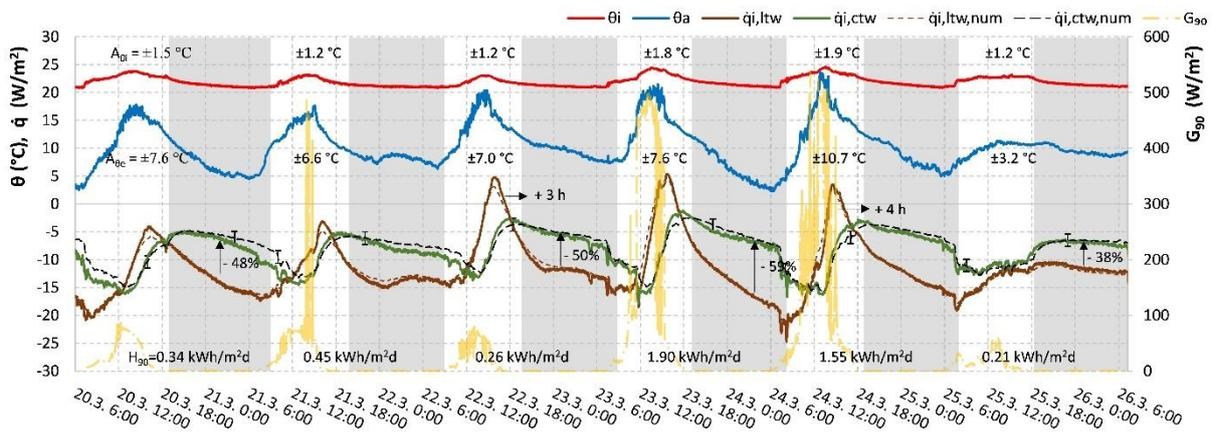
**Fig. 4.** In-situ measured solar radiation, air temperatures and inner surface heat flux for laminated timber (*ltw*) and composite timber wall (*ctw*) and calculated heat flux of composite timber wall ( $d_{VIP} = 6 \text{ mm}$ ,  $d_{PCM} = 10 \text{ mm}$ ).
