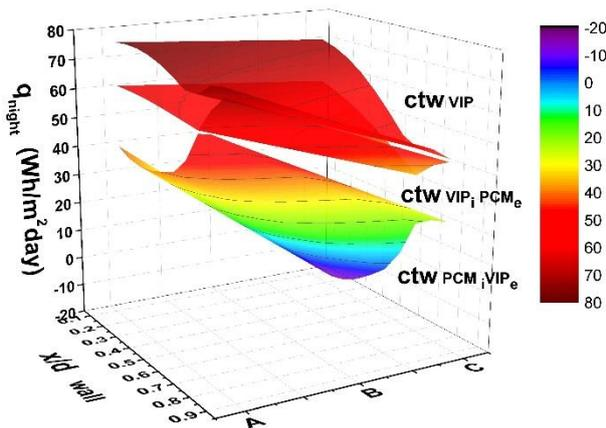
**Fig. 8.** Composite timber façade walls' heat losses in the night-time period (from 19:00 until 8:00) according to the relative position of VIP or VIP/PCM panel in the composite wall and different indoor boundary conditions;  $H_{90} = 2.5$  kWh/m<sup>2</sup>day.
