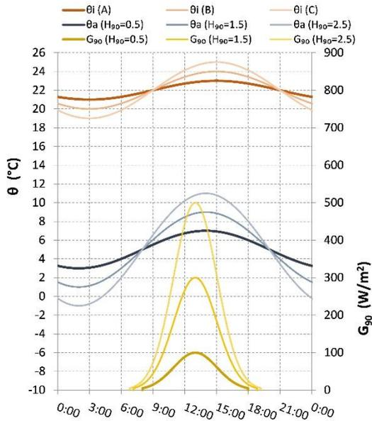
**Fig. 5.** Indoor and outdoor temperature and solar radiation boundary conditions adopted for analysis
