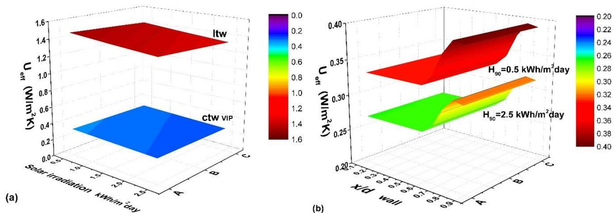
**Fig. 6.**  $U_{eff}$  values of laminated and composite timber wall with integrated VIP panel ( $ctw_{VIP}$ ) according to outdoor and indoor dynamic boundary conditions (a) and  $U_{eff}$  values of  $ctw_{VIP}$  according to the relative position of VIP panel in the composite wall at different boundary conditions (b)
