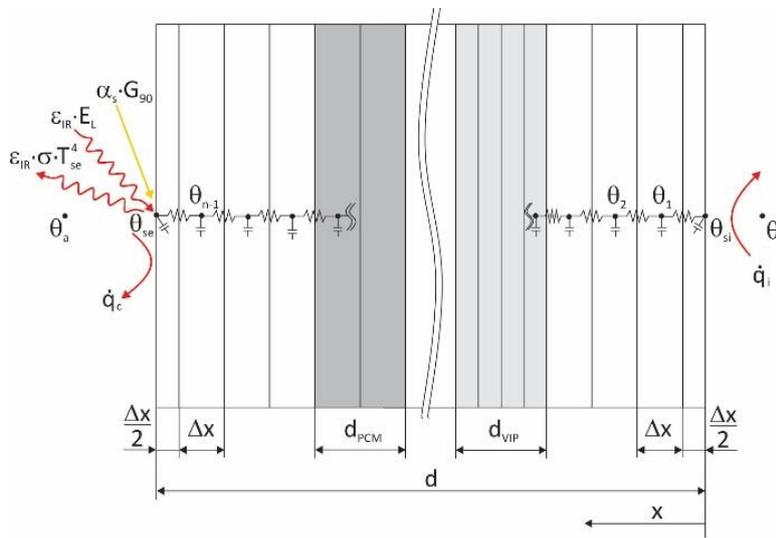
**Fig. 2.** Schematic of the nodal network and heat fluxes considered in the mathematical model of a thin composite timber façade wall with PCM and VIP layer.
