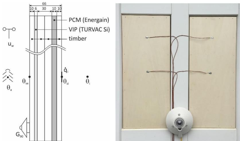
**Fig. 3.** Schematic of composite timber wall with VIP and PCM layer used in the experiment and the experimental setup (left) and close view (outer side) of comparative in-situ measurements of laminated timber and composite timber wall (right)
