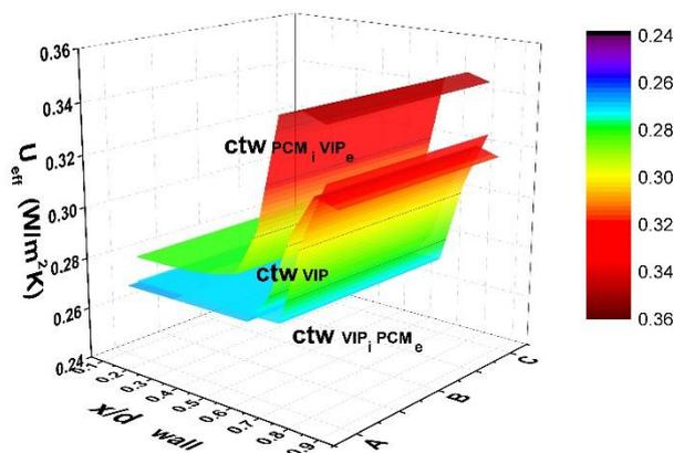
**Fig. 7.**  $U_{eff}$  values of composite timber walls with integrated VIP panel and integrated VIP/PCM panels according to the relative position of VIP or VIP/PCM panel in the composite wall and different indoor boundary conditions;  $H_{90} = 2.5$  kWh/m<sup>2</sup>day.
