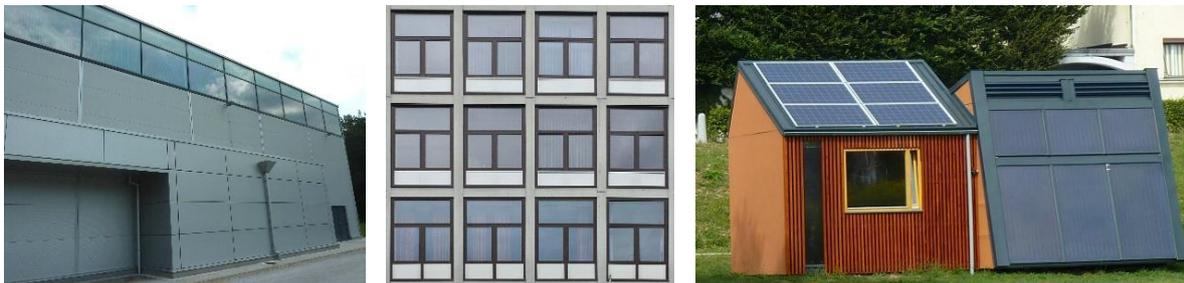
**Fig. 1.** Buildings made of thin, lightweight building envelope elements: metal façade (left), thin prefabricated opaque/transparent walls (middle), mobile homes (right).
