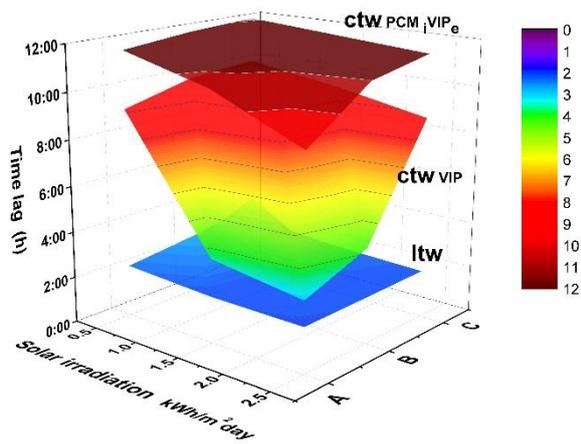
**Fig. 9.** Time lag of periodic heat wave propagation for laminated timber wall and for composite timber façade walls with VIP and VIP/PCM panels at optimal location within  $ctw$ .
